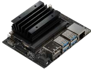
Figure 13: Nvidia Jetson Nano (Source: Franklin)
