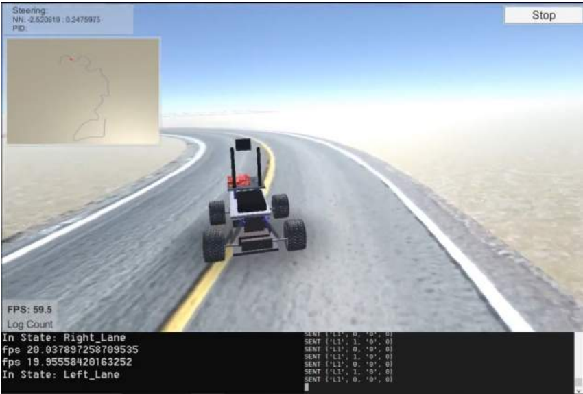
Figure 111: Simulator testing: Returning to left lane behaviour
