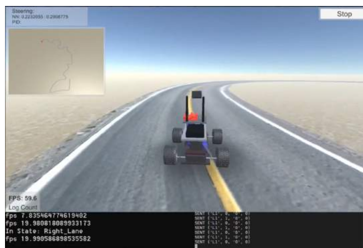
Figure 110: Simulator testing: Switching to right lane behaviour
