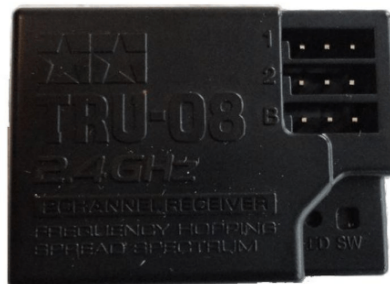
Figure 9: Wireless receiver (Source: RC-Hobbies)
