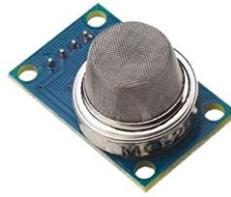
Slika 38: MQ-2 digitalni senzor plina (Preuzeto sa: <https://images-na.ssl-images-amazon.com/images/I/51S1R01YqUL. SX342 .jpg>)
