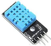
Slika 37: DHT11 digitalni senzor temperature i vlage (Preuzeto sa: [https://images-na.ssl-images-amazon.com/images/I/31EM6oovwLL.\\_SX466\\_.jpg](https://images-na.ssl-images-amazon.com/images/I/31EM6oovwLL._SX466_.jpg))
