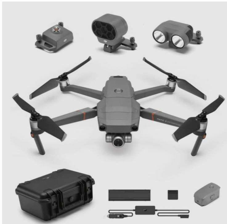
Slika 4: DJI Mavic2 Enterprise dron s nastavcima Beacon, Speaker i Spotlight (Izvor: [drone-works.com](http://drone-works.com))
