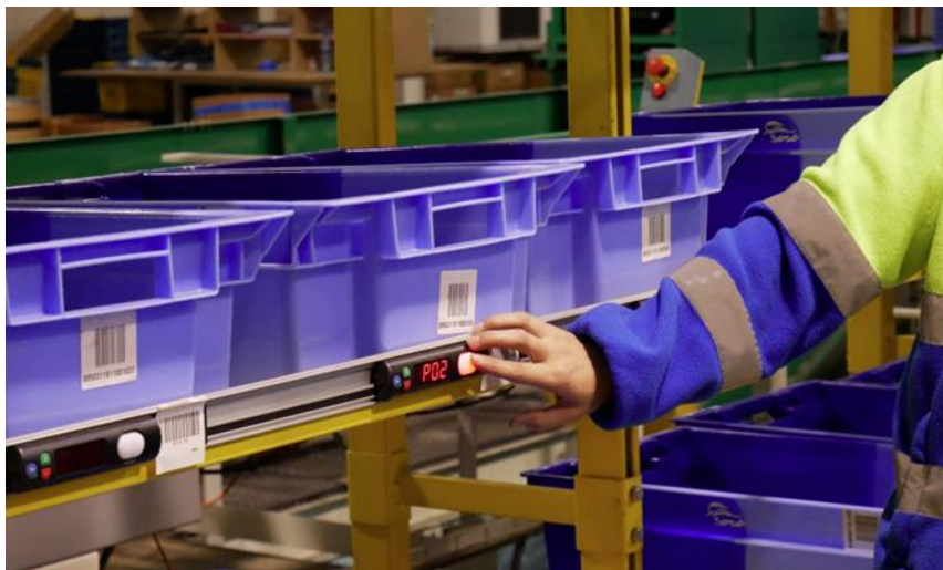
Slika 5: Primjer Pick to Light uređaja u skladištu (Izvor: Pick to light, n.d.; dostupno na: https://www.picktolightsystems.com/en/picking-products/pick-by-light )
