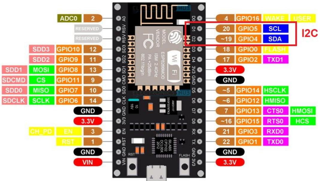
Slika 8. I2C pinovi na ESP8266 (Izvor: ElectronicsHub.com)
