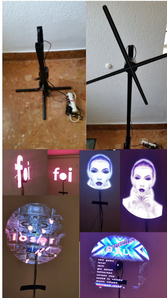
Figure 3.1: Developed volumetric 3D display
