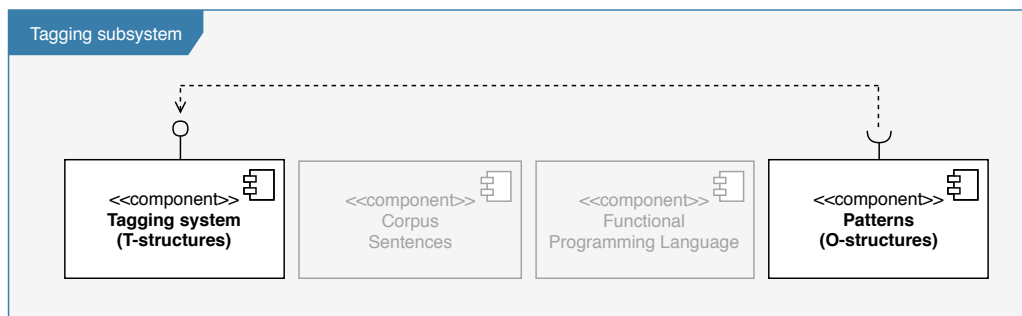
Figure 11: Conceptual model of a tagging subsystem
