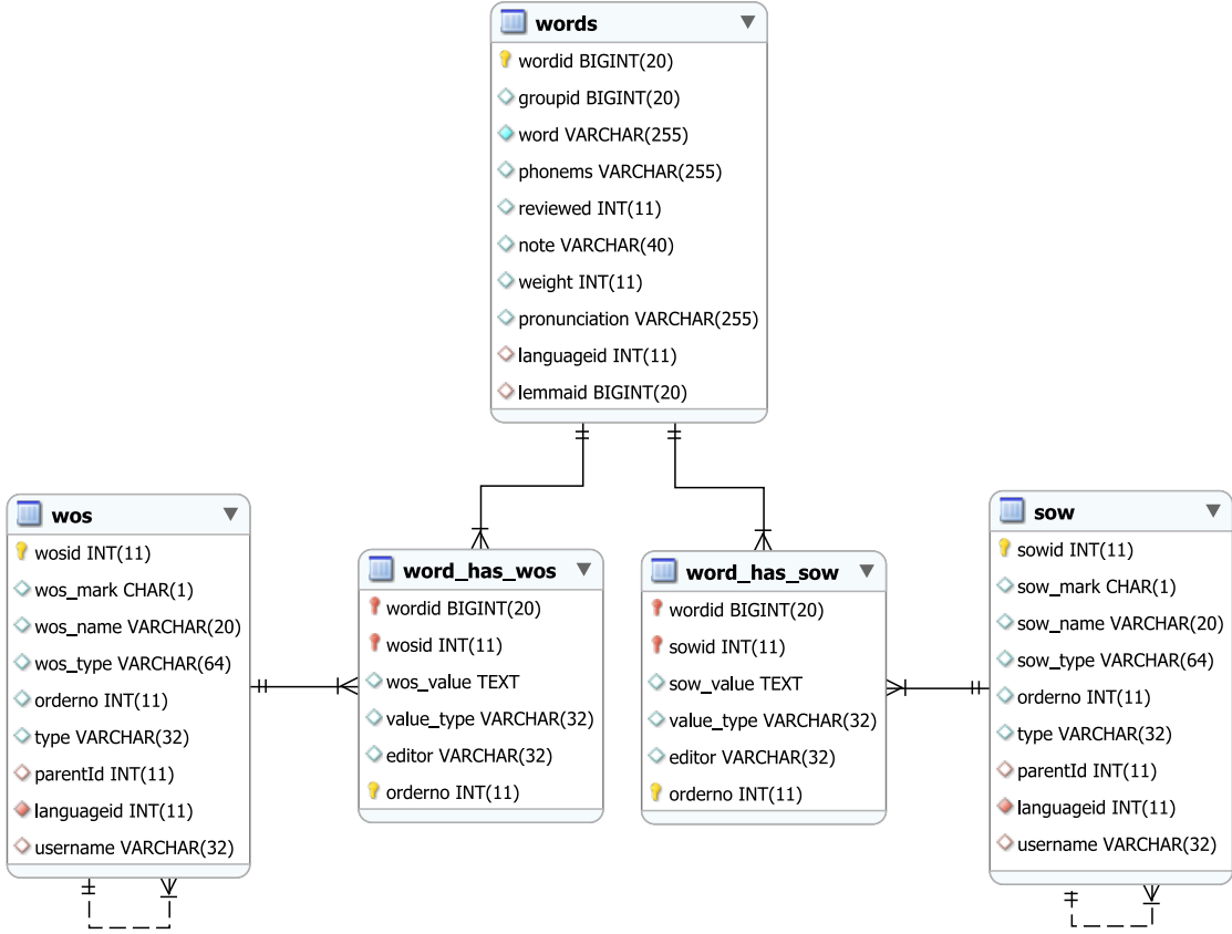
Figure 15: Database model of word tagging
