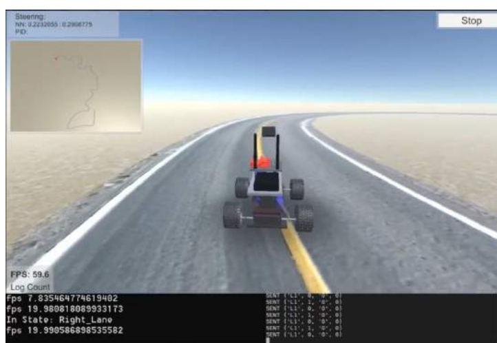
Figure 110: Simulator testing: Switching to right lane behaviour
