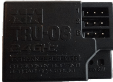
Figure 9: Wireless receiver (Source: RC-Hobbies)
