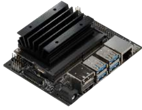
Figure 13: Nvidia Jetson Nano (Source: Franklin)
