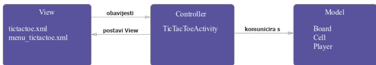
Slika 3: TicTacToe - Model-View-Controller (Maxwell, 2017)
