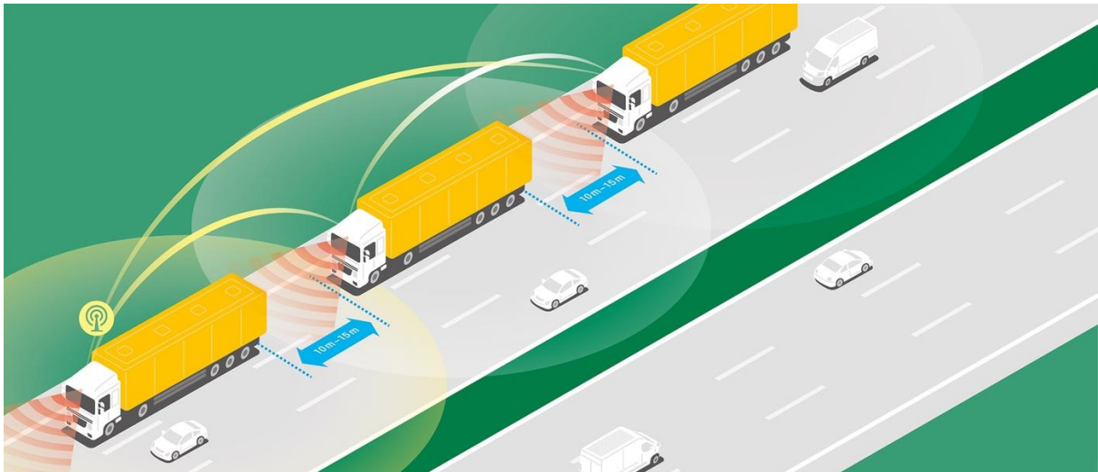
Figure 4: Visualization of Truck Platooning; Source: [6]
