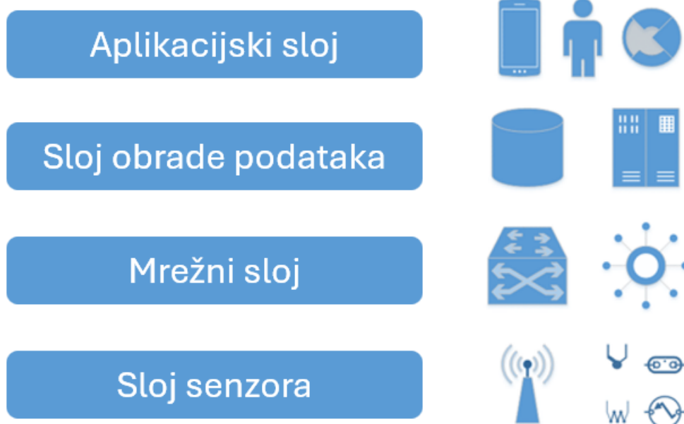
Slika 7: Arhitektura IoT-a Izvor: https://www.hiotron.com/iot-architecture-layers/
