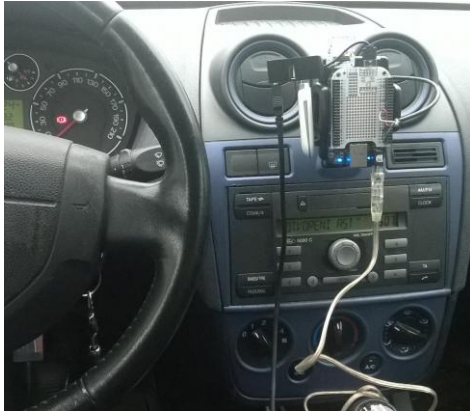
Fig. 4. The automobile embedded system with attached GPS module and mobile Internet module, connected to the automobile OBD-II interface.
