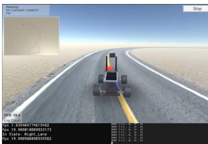
Figure 110: Simulator testing: Switching to right lane behaviour
