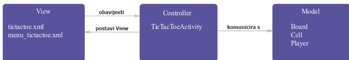
Slika 3: TicTacToe - Model-View-Controller (Maxwell, 2017)
