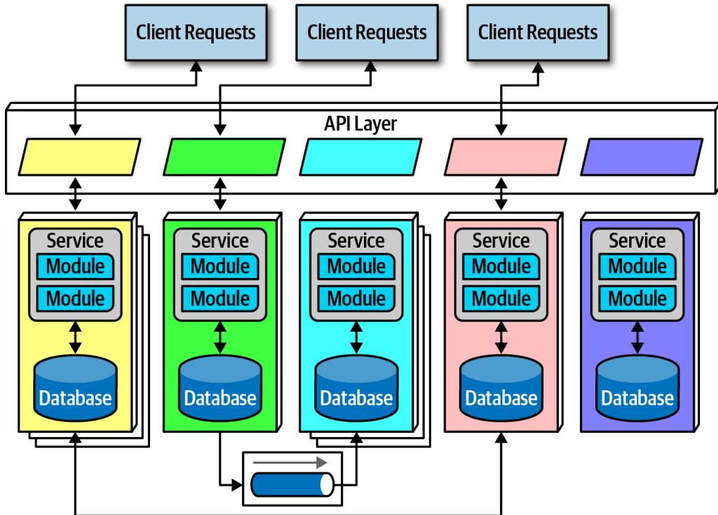
Slika 16: Mikroservisni arhitekturalni stil (*Richards & Ford, Fundamentals of Software Architecture, 2020*)
