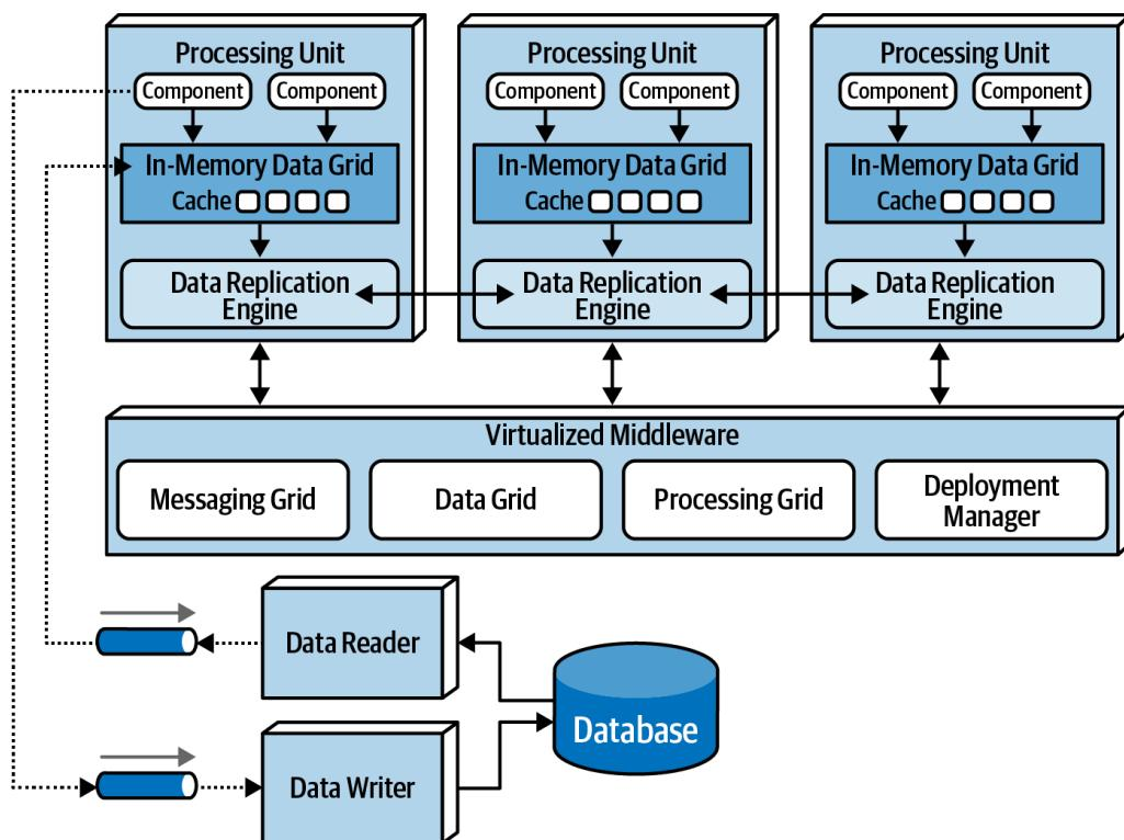
Slika 14: Standradni stil temeljen na prostoru (*Richards & Ford, Fundamentals of Software Architecture, 2020*)
