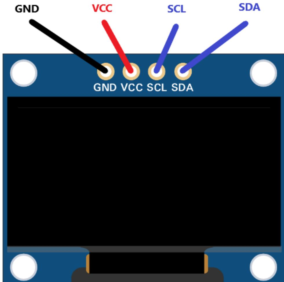
Slika 7: OLED SSD1315 pinout (Izvor: autor, 2023)
