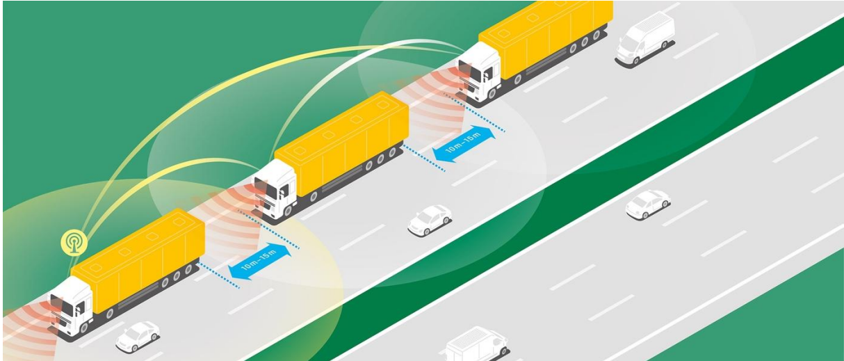
Figure 4: Visualization of Truck Platooning; Source: [6]
