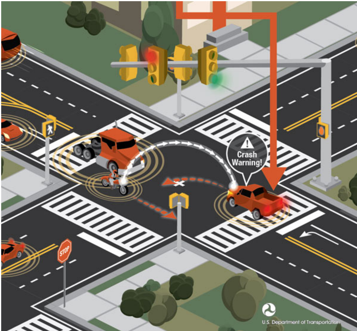
Figure 3: Left-Turn Warning Visualization; Source: [5]
