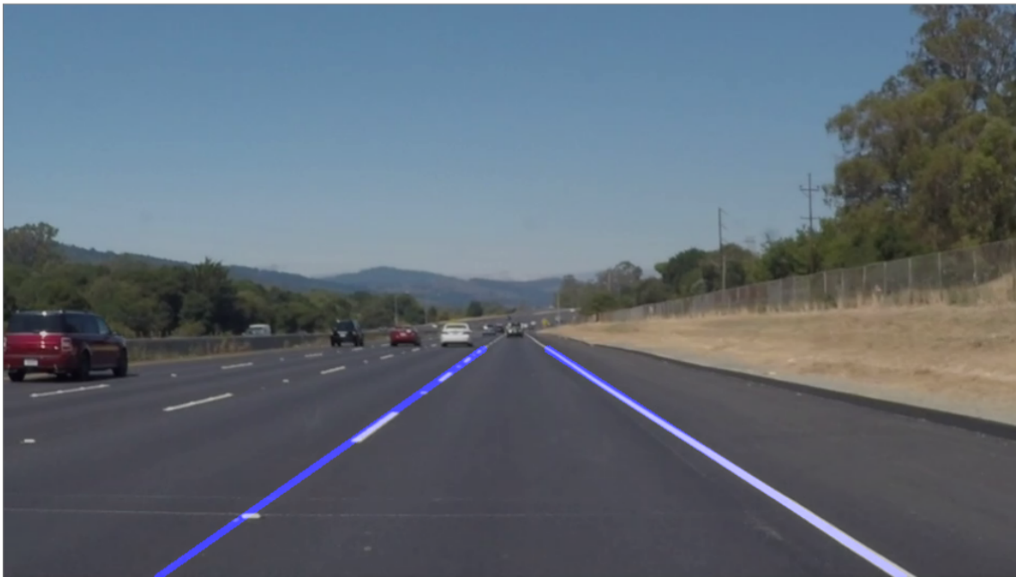
Figure 5.3: Lane line as detected by the algorithm [38]
