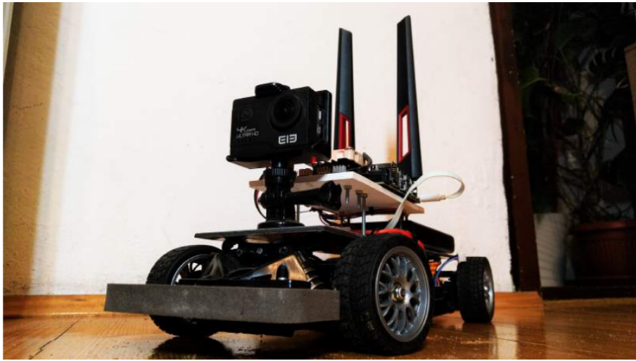
Figure 5.1: The assembled car [45]
