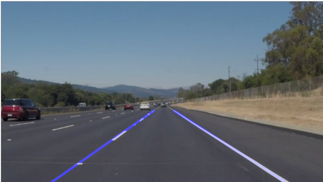
Figure 5.3: Lane line as detected by the algorithm [38]
